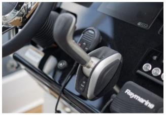
2024 Williams Jet Tenders Dieseljet 505 control panel with steering wheel and throttle.
