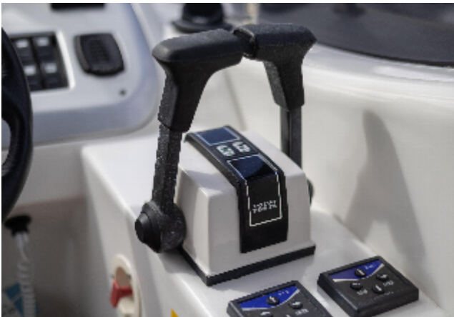
Volvo Penta throttle controls on 2006 Sessa Marine C35 boat dashboard.
