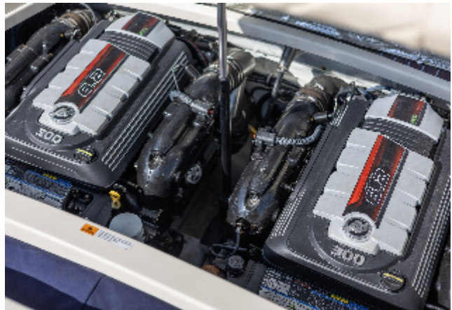
2017 Chris-Craft Launch 30 engine compartment with dual 6.2L Mercury engines.
