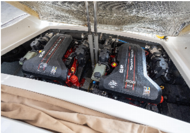
Engine compartment of 2013 Chris-Craft Corsair 28 Heritage Edition with Volvo Penta V8 engines.
