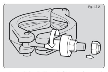
• Open up the Fast Fit clamp and offer the gearbox up to the above deck unit, sliding the shaft into the gearbox. Ensure the drive key is in place.
