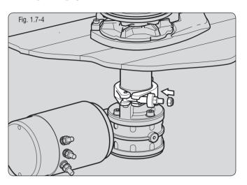
Tighten up the bronze nut to 15 Nm (11 lb/ft) before adding the Nyloc nut. Tighten the Nyloc nut up behind the bronze nut.
