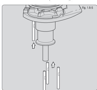
• Fully screw the four mounting studs into the base of the windlass. Screw the studs into the base finger tight, with the flats towards the base as shown (Fig 1.6-5).
