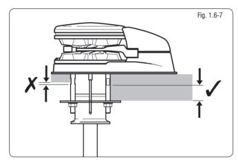
• Place the base mat in position on the deck, optionally, apply a suitable sealant to the base of the windlass, any mounting pad or around the studs.
