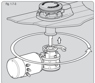
• Place the gearbox up the shaft and rotate it into a suitable position before finally pushing home onto the location dowels.
