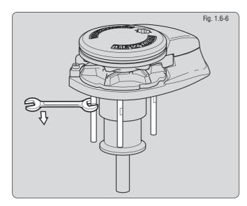
• Next, using a 7 mm (1/4") spanner on the flats, tighten the studs until they bottom out in their holes. Do this to each of the studs in turn.
