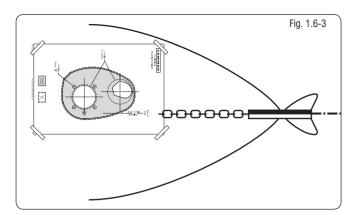
• Place the mounting template on the deck or mounting pad in the desired position for the windlass and hold it in place using adhesive tape.
