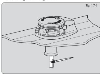
• Remove the nyloc nut from the end of the Fast Fit clamp bolt and screw the bronze nut up to the end of the thread.
