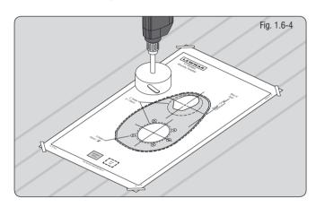
Using a 10 mm (<sup>3</sup>/<sub>8</sub>") diameter drill, make the five holes for the mounting studs and sensor. With a 75 mm (3") diameter hole saw, make two holes for the rode and down tube to pass through.
